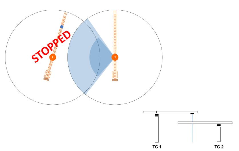
Trolley sensor fault on the higher crane
