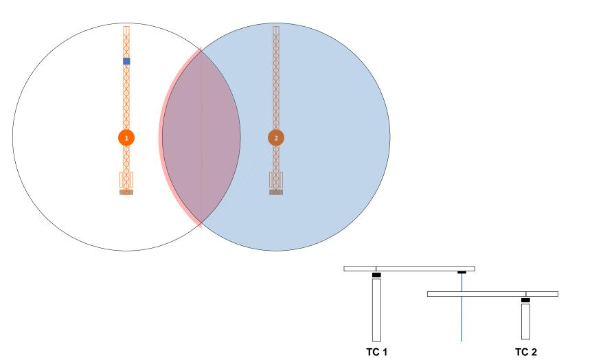
System on the lower crane bypassed
