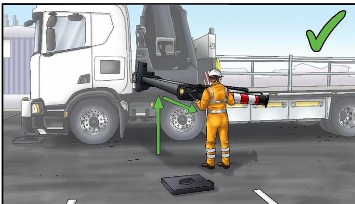
Manually operated swing-up stabilisers are not hydraulically (or otherwise) powered. They require the Operator to physically push the stabiliser leg into its correct stowage position, typically aided by a gas spring. Locking functions must be disengaged/released before the swing-up or swing-down movement is possible.
