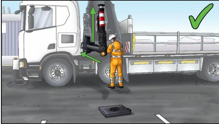
Such systems may take various forms. E.g., preventing full retraction of the stabiliser unless it is in an upwardly vertical position.
